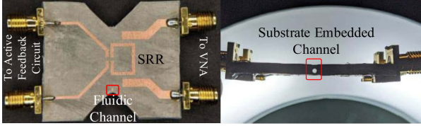
FIGURE 22. Microfluidic channel embedded within the sensor substrate by micro-milling a cavity within the dielectric substrate of the sensor in [66]. Reprinted with permission from [66]; copyright 2022 IEEE.
